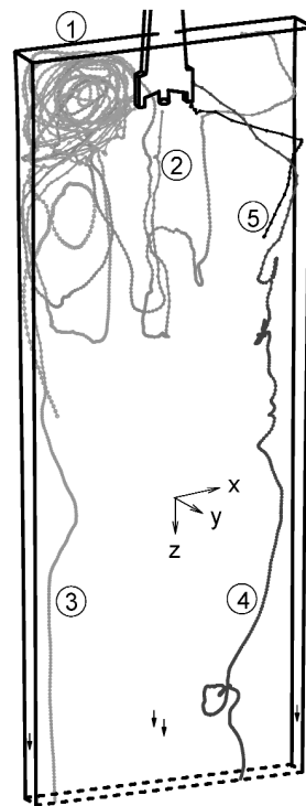
Fig. 11—Predicted representative particle trajectories in an actual steel caster (case 2-S).
